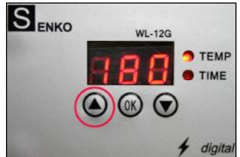
Select with arrows temperature required, (Normally 180°C) Left arrow select Up. Right arrow select Down
