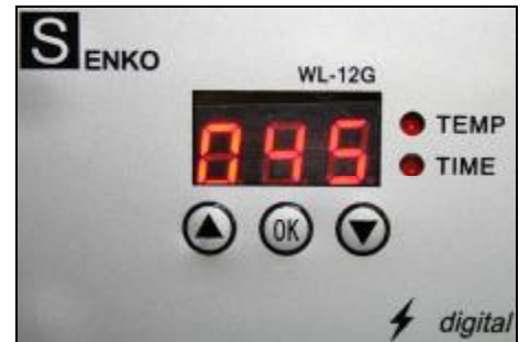
Press OK button again, The program will stay in memory of the control board and the temperature starts to rise
