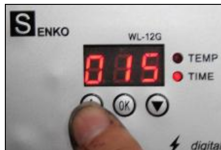
Select with arrows time required, (normally 15 seconds)
