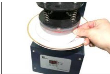
Place the transfer ink side down onto plate
