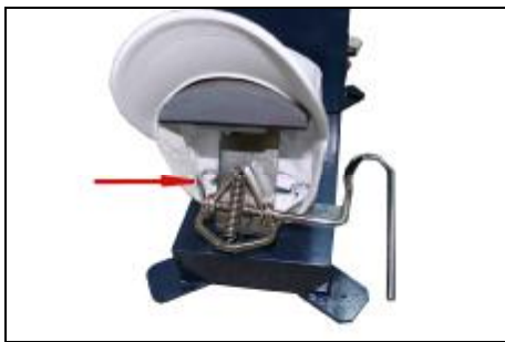
Clip the cap into the silicon heater and flat the cap
