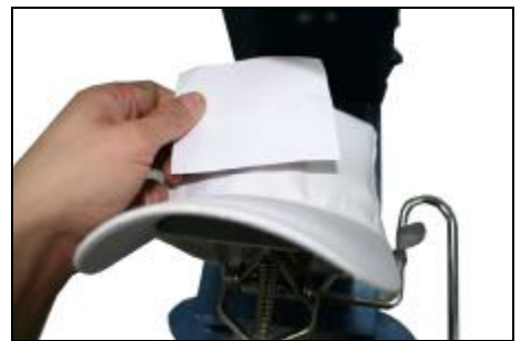
Place the transfer ink side down onto the cap
