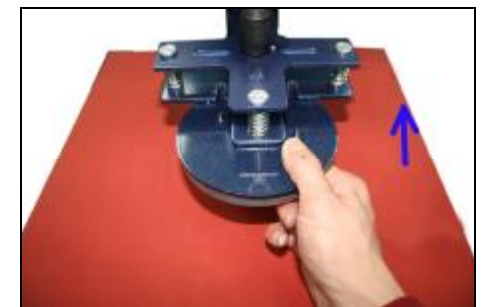
Push the platen to the end, no need to lock screw cap, since it is with magnet.
