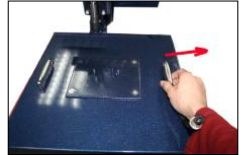
Bring up the heat platen directly
