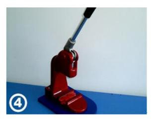
**Step 3:** Open the box for moulds and install the upper mould as the picture 5 & 6 shown; please aim at the right azimuth as red drawn
