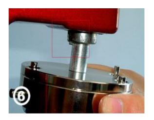
**Step 4:** Boost up the upper mould and insert the bottom mould from left to right; then put the bolt in the left as the picture 7&8 shown.
