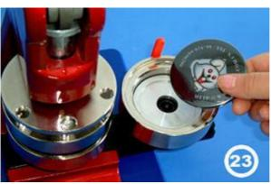
**Step 9:** If you want to make a Cartoon Button, please put the plastic shell onto right mould to make it as picture 24, 25, 26, 27 shown.
