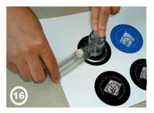
**Step 7:** Put the pin, paper and plastic film in turn (if the paper is thick as the photo paper, please one plastic film is OK; if the paper is thin, two plastic films will be better) onto the left bottom mould, then press the left mould as picture 17& 18 shown.
