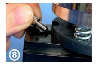
**Step 5:** Move the bottom mould and press the handle to test the pressure as picture 9, 10, 11 shown.
